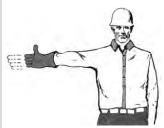
BOOM UP AND LOWER THE LOAD
